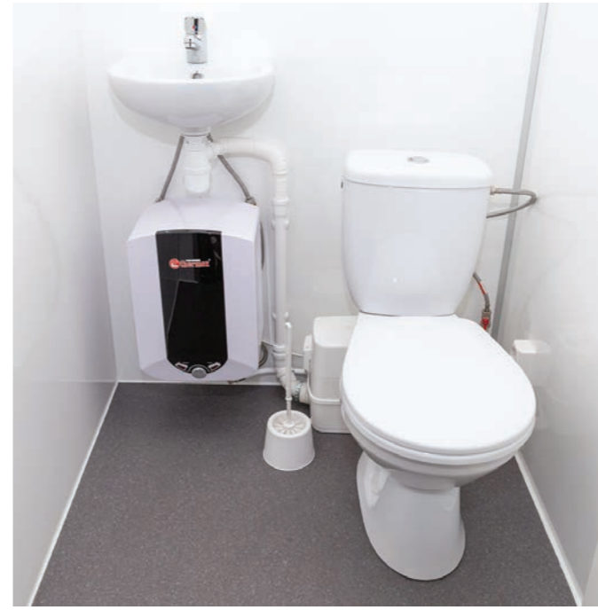
This toilet system connects to the external sewer. Includes a ceramic toilet, sink, boiler 10L, grinder. Fresh water - plastic quick connector 3/4", outlet for waste water BEM connector 32mm inside and 39mm outside.
