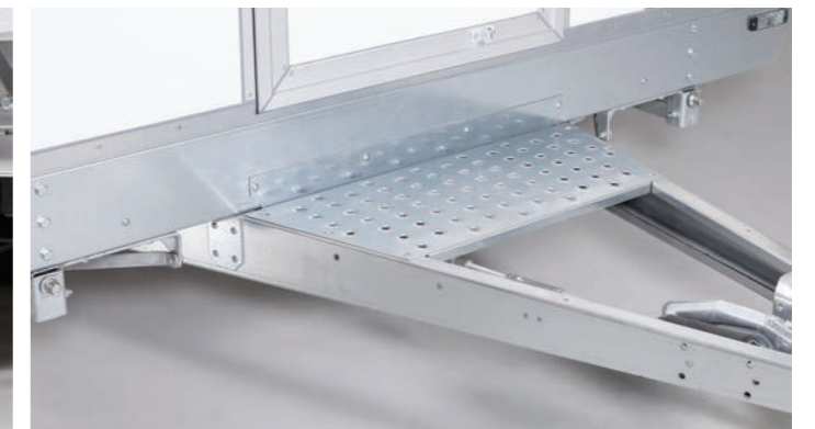
Fixed stairs on the draw bar.
