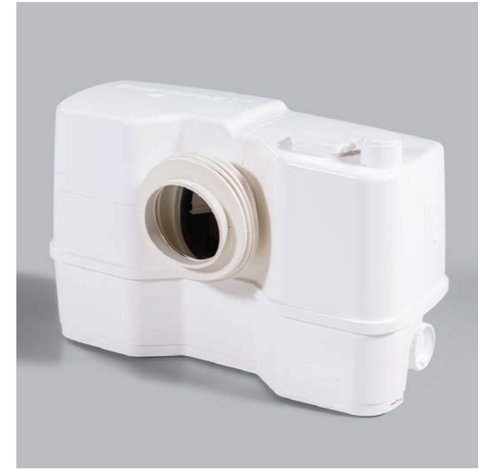
Grinder deals with the waste coming from the sink and toilet. The device grinds waste into a semi-liquid mixture and pumps it through a hose to the central sewer system.
