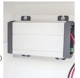
Battery charger ensures that battery is always fully loaded.
