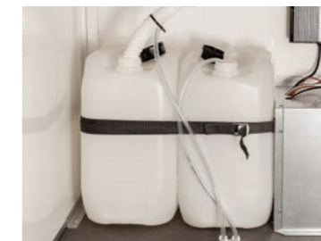
Fresh water canister (30L) and waste water canister (30L).
