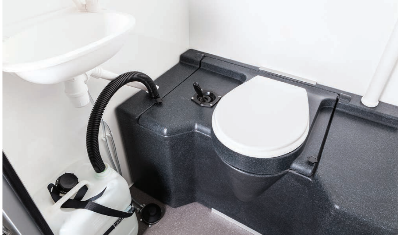
300L tank toilet with a hand pump. Plastic sink and 25l canister with a foot pump. Easy to fill the water canister and to see how much water is left. When the mobile office is not in active use the canister needs to be emptied when temperature drops below 0 C. In temperatures below 0 C it is recommended to add antifreeze fluids into the tank.
